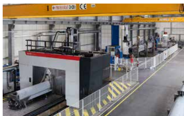
Telemond | Automatic welding line for telescopic booms
